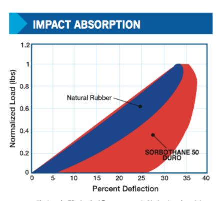
Hysteresis (Mechanical Energy converted to heat each cycle)
